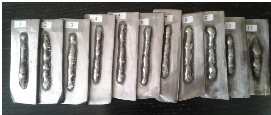
Fig. 2. Samples surfaced by plasma surfacing at various modes
