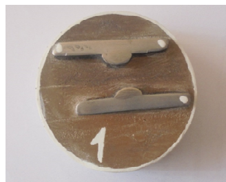
Fig. 3. Prepared micro-sections surfaced by plasma powder method with different content of tungsten carbide and pressed into epoxy resin
