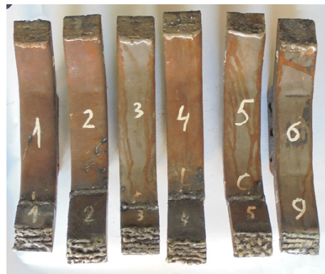
Fig. 4. Restored chisels of Gaspardo Artiglio deep-ripper
